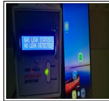
Figure 8: Automatic gas detection system showing no leakage detected
