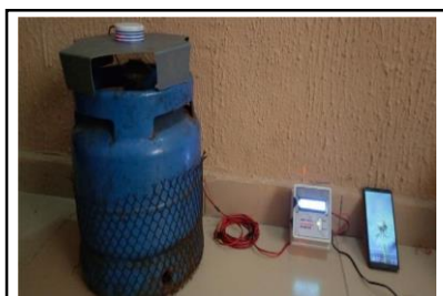
Figure 7: Automatic gas detection set up
